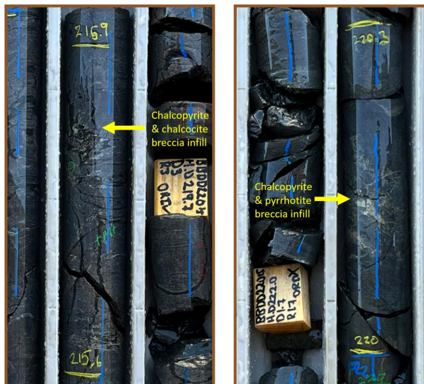
Figure 1. Small crackle breccia zones within Bambino drillhole BBDD22015 are infilled with chalcopyrite and trace chalcocite (<2% sulphides on the left) and chalcopyrite and pyrrhotite (~5% total sulphides on the right).
